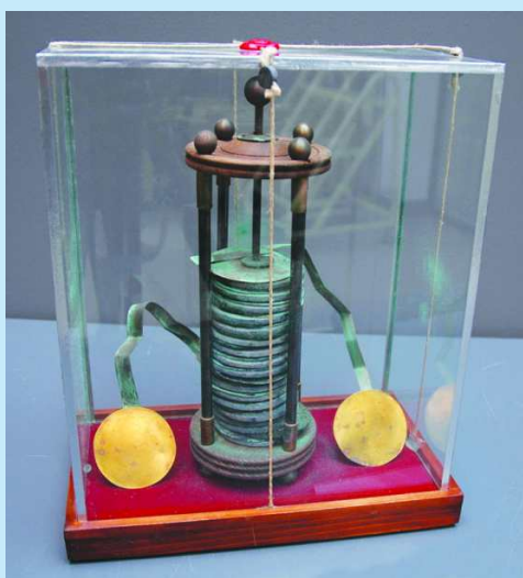
A Voltaic pile
