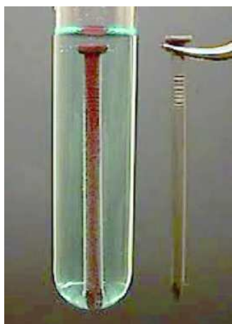
fig-11(a): Iron nail dipped in copper sulphate solution
